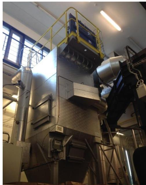
Continuously operating pilot-scale waste incinerator with filtration unit
