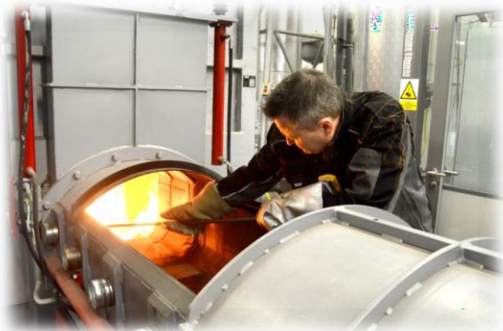
Continuously operating pilot-scale waste incinerator
